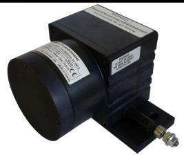
The AWP series are wire potentiometric position transducers that turn a linear motion into a resistance variation. They are made of a precision rotating potentiometer operated by a, winding or unwinding, stainless steel wire. Optionally other stroke lengths, cable length and socket connector can be requested.
