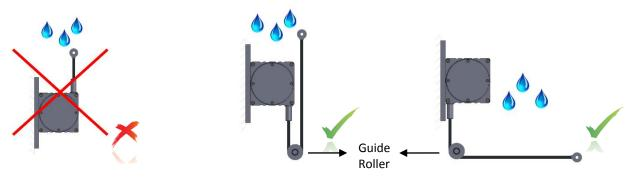
4. The wire should not be pulled in angular. If needed, please use guide rollers.
