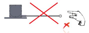
2. The wire encoder must be mounted vertically in position, not be horizontally.
